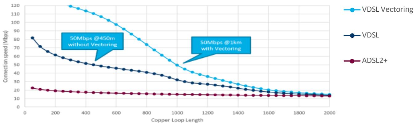
Vectoring relies on interaction between our DSLAM and Customer CPE. For example, downstream vectoring works as follows:
