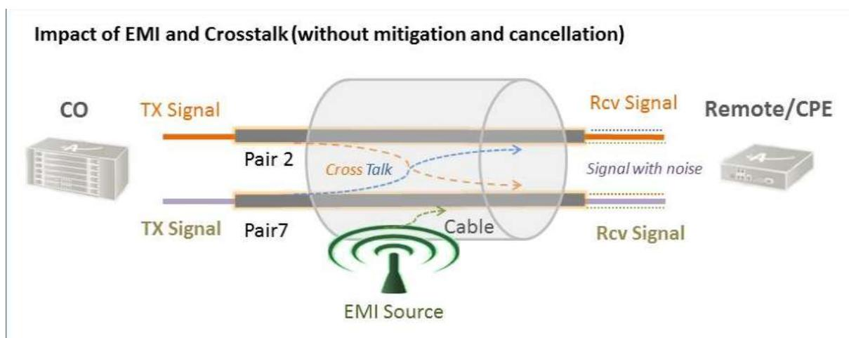
This crosstalk is influenced by the proximity, level and number of adjacent signals. VDSL2 is particularly susceptible to far end crosstalk due to its higher frequencies resulting in greater signal loss over shorter transmission distances. This higher attenuation of the signal causes VDSL2 bandwidth decreases significantly the more VDSL2 services there are in a common cable sheath.
