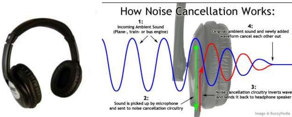
The noise cancellation technology in headphones, for example, has few variables to address as it suppresses interference in the audio band (20 kHz). They pick up ambient noise (via an external-facing microphone) and generate an anti-noise signal that compensates or neutralises the ambient noise at the ear.
