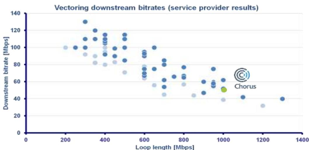
Vectoring is only effective if all lines in a cable bundle are fed by the same DSLAM. This makes vectoring unsuitable for unbundled areas or where cable pairs are spread across multiple DSLAMs.
